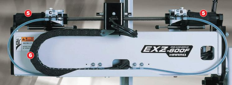
Smooth takeout of sprues with the servo-driven vertical axis
